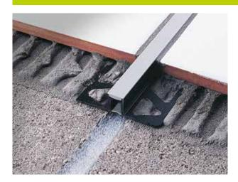
Conceived to subdivide large tile bays, COFLEX CA movement joints in co-extruded synthetic resin are composed of rigid, perforated anchoring flanges and a durable, soft upper surface which is resistant to mildew, bacteria, weathering, corrosion, wear and UV rays. Suitable for indoor and outdoor applications; the profile section provides limited protection to the tile edge. Ideally used in retail shops, hotels, sports facilities and schools.
